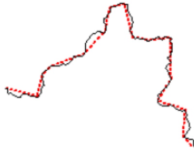
Fig. 4. Map generalization could smooth the water border (taken from map generalization document)
